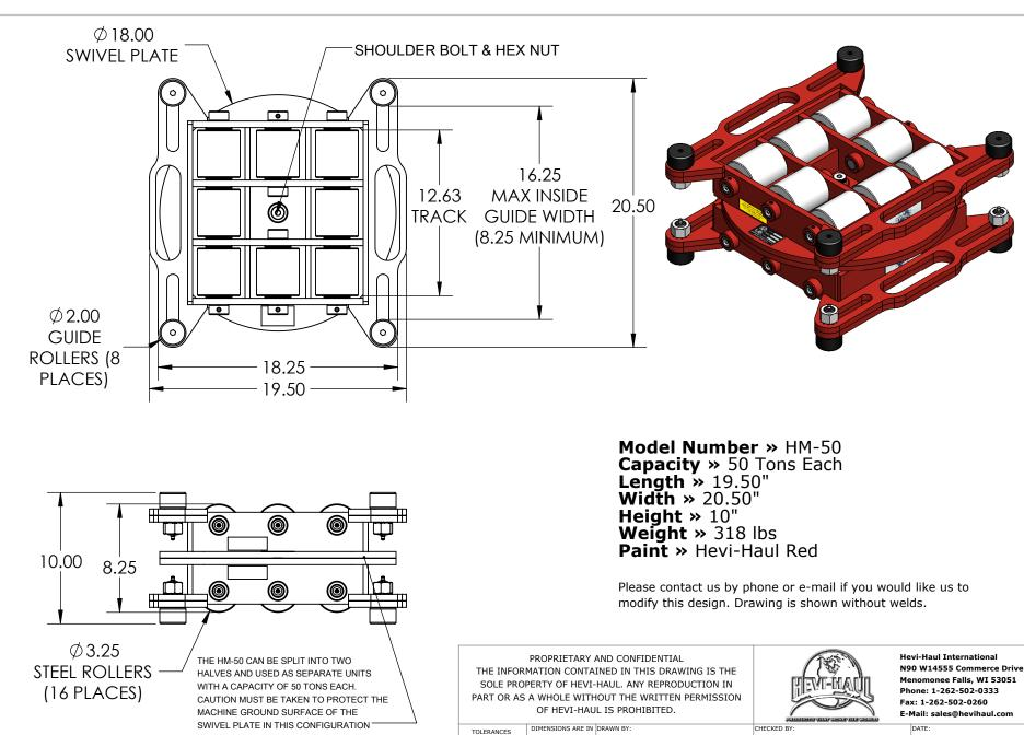
INCHES 1/26/2017 UNLESS NOTED G.L. Schneider DO NOT SCALE BREAK SHARP EDGES DRAWING HM-50 - Specification Sheet X.XX +/- 0.030 THIRD ANGLE PROJECTION x.xxx +/1 0.005 DRAWING NUMBER: REVISION: SCALE ANGLE +/- 0.5\* HM-50 1:8 MACHINE 125
