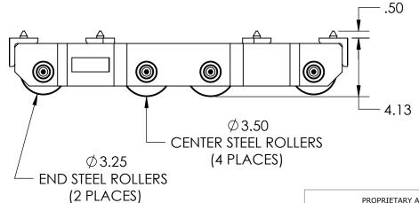
Model Number » UM-HD-75 Capacity » 37.5 Tons Each Length » 23.75" Width » 11" Height » 4.125" Weight » 97 lbs Paint » Hevi-Haul Red
