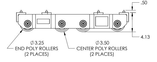
Model Number » UM-HD-75-P Capacity » 20 Tons Each Length » 23.75" Width » 11" Height » 4.125" Weight » 74 lbs Paint » Hevi-Haul Red
