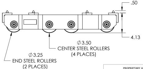
Model Number » UM-HD-50 Capacity » 25 Tons Each Length » 23.75" Width » 11" Height » 4.125" Weight » 97 lbs Paint » Hevi-Haul Red
