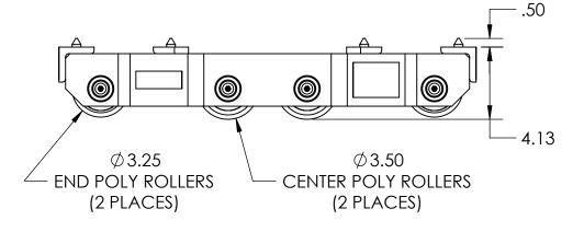
Model Number » UM-HD-50-P Capacity » 20 Tons Each Length » 23.75" Width » 11" Height » 4.125" Weight » 74 lbs Paint » Hevi-Haul Red
