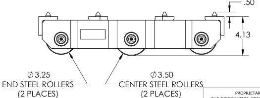
Model Number » UM-HD-30 Capacity » 15 Tons Each Length » 19.50" Width » 11" Height » 4.125" Weight » 70 lbs Paint » Hevi-Haul Red
