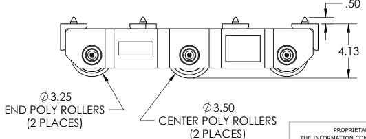
Model Number » UM-HD-30-P Capacity » 15 Tons Each Length » 19.50" Width » 11" Height » 4.125" Weight » 56 lbs Paint » Hevi-Haul Red
