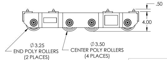
Model Number » UM-HD-15-P Capacity » 7.5 Tons Each Length » 23.50" Width » 10.50" Height » 4" Weight » 58 lbs Paint » Hevi-Haul Red
