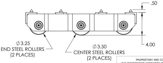
Model Number » UM-8 Capacity » 4 Tons Each Length » 19.25" Width » 10.50" Height » 4" Weight » 55 lbs Paint » Hevi-Haul Red
