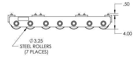
Model Number » TDM-7 Capacity » 12.5 Tons Each Length » 29.75" Width » 6.5" Height » 4" Weight » 121 lbs Paint » Hevi-Haul Red
