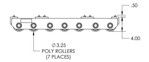
Model Number » TDM-7 Capacity » 12.5 Tons Each Length » 29.75" Width » 6.5" Height » 4" Weight » 100 lbs Paint » Hevi-Haul Red
