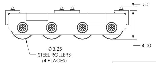
Model Number » TDM-4 Capacity » 7.5 Tons Each Length » 17" Width » 6.50" Height » 4" Weight » 62 lbs Paint » Hevi-Haul Red
