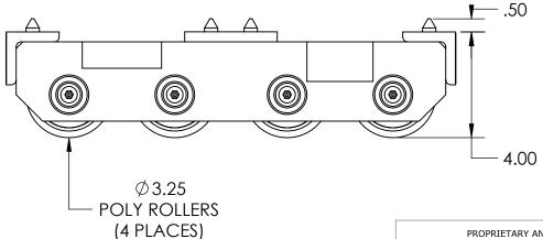
Model Number » TDM-4-P Capacity » 7.5 Tons Each Length » 17" Width » 6.50" Height » 4" Weight » 50 lbs Paint » Hevi-Haul Red
