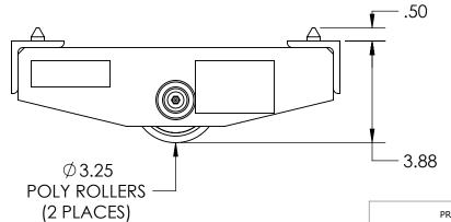
Model Number » TD-35 Capacity » 3 Tons Each Length » 12.50" Width » 10.50" Height » 3.875" Weight » 29 lbs Paint » Hevi-Haul Red
