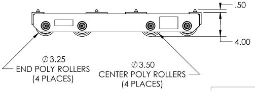
Model Number: HD-15-P Capacity » 10 Tons Each Length » 27.75" Width » 10.50" Height » 4" Weight » 81 lbs Paint » Hevi-Haul Red
