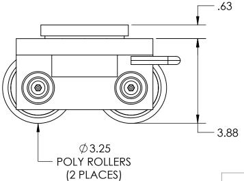
Model Number » CS-5-P Capacity » 2.5 Tons Each Length » 8.125" Width » 6" Height » 4.5" Weight » 24 lbs Paint » Hevi-Haul Red
