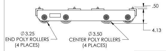
Model Number: BB-100-P Capacity » 20 Tons Each Length » 28" Width » 12" Height » 4.125" Weight » 121 lbs Paint » Hevi-Haul Red
